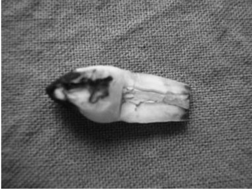
Figure 1. Dye penetration of amalgam filling.
