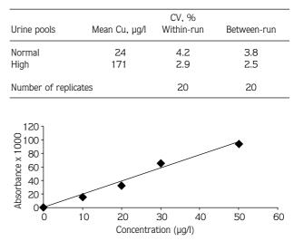
Figure 1. Linearity of the new photometric method.
