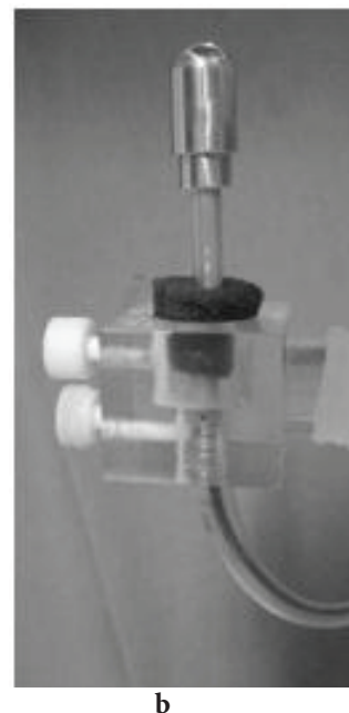
Figure 3. Designed PMMA miniphantom: a) experimental setup, b) brass miniphantom.
