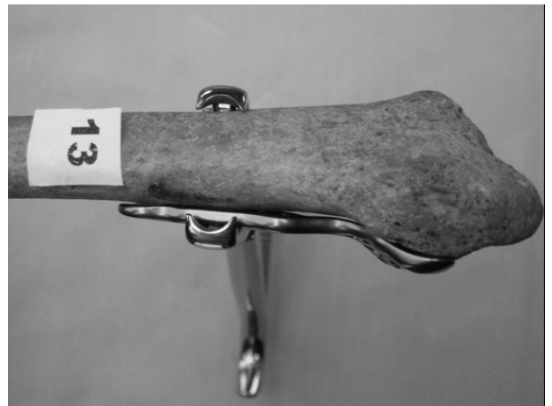
Figure 6. Acumed Acu-loc Standard plate is more suitable for radius number 13.
