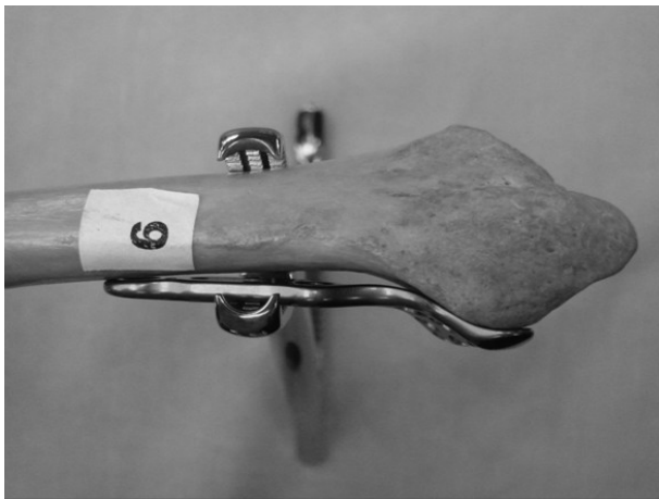
Figure 5. Acumed Acu-loc Standard plate does not fit to radius number 9.
