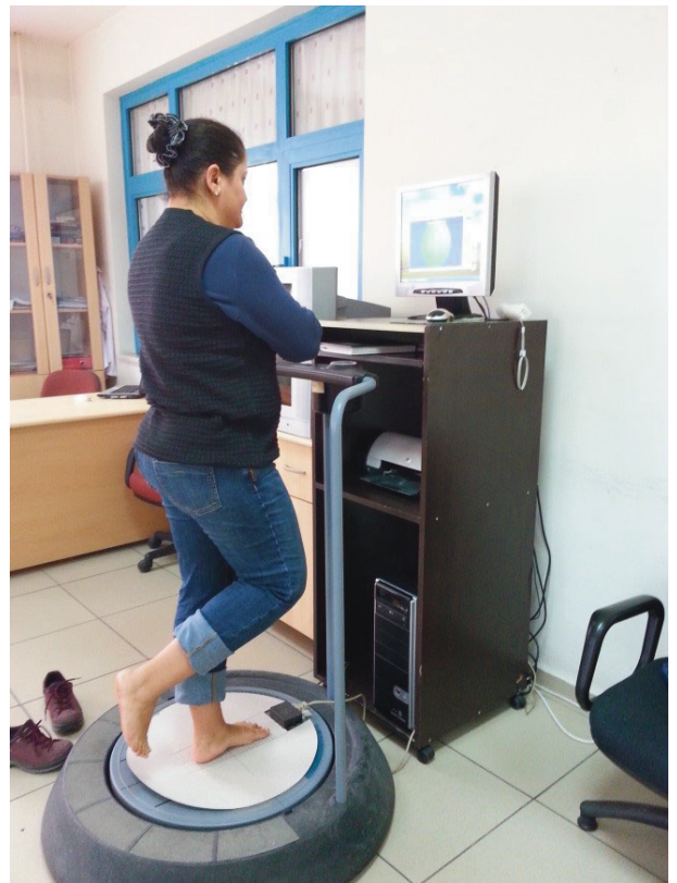
Figure 2. The measurement of the static equilibrium index with the Kinesthetic Ability Trainer 3000.
