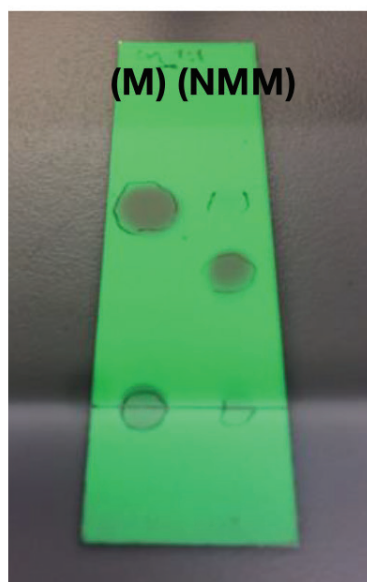
Figure 5. Thin layer chromatography of maleimide and N-methylolmaleimide.
