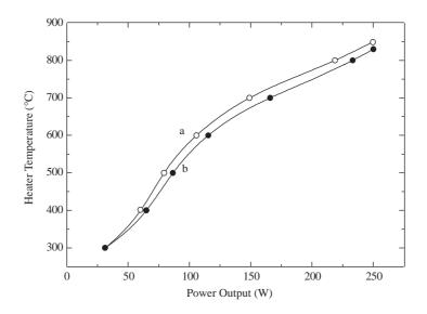
Figure 2. Heater surface temperature versus applied power to the filament. a)  $Ar + O_2$  gas mixture pressure is 1  $\mu$ Torr; b)  $Ar + O_2$  gas mixture pressure is 200 mTorr. The lines are for the eye.
