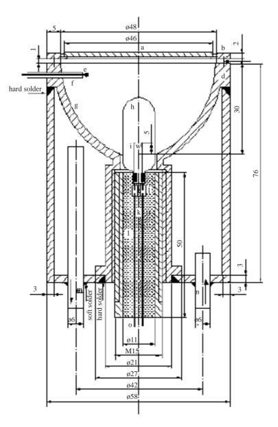
Figure 1. Block diagram of the heater (all dimensions are in millimeters): a) Ni Holder; b) Stainless steel ring; c) Four Ni-Cr wire supports; d) Brass block; e) K-type (chromel-alumel) thermocouple; f) Ceramic tube; g) Ni-Cr plated parabolic cavity; h) 250 W halogen bulb; i) Bulb filament at the focus of the paraboloid cavity; j) Crimped copper tubing; k) Copper wires; l) Cement filled bulb holder; m) Cooling water outlet; n) Cooling water inlet; o) Electrical feedthroughs.
