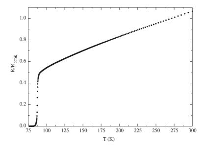
Figure 4. Normalized electrical resistance versus temperature for the prepared  $YBa_2Cu_3O_{7-\delta}$  thin film.
