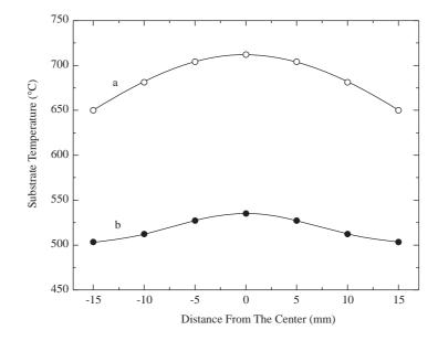
Figure 3. Variation of the temperature on the holder surface at  $Ar + O_2$  gas mixture pressure of 1  $\mu$ Torr. a) Set temperature is 700 °C; b) Set temperature is 525 °C. The lines are for the eye.
