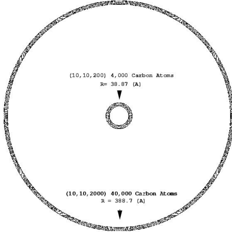
Figure 1. Starting structure of two toroids with different radii, the smallest stable toroid and the largest toroid used in our calculation.
