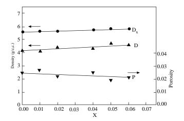
Figure 4. The density and porosity as a function of Sm content x.
