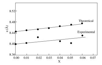
Figure 2. The theoretical and experimental lattice parameters as a function of Sm content x.
