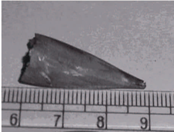
Figure 1. \text{Sb}_2\text{Se}_3 crystal grown by Bridgman Stockbarger method.
