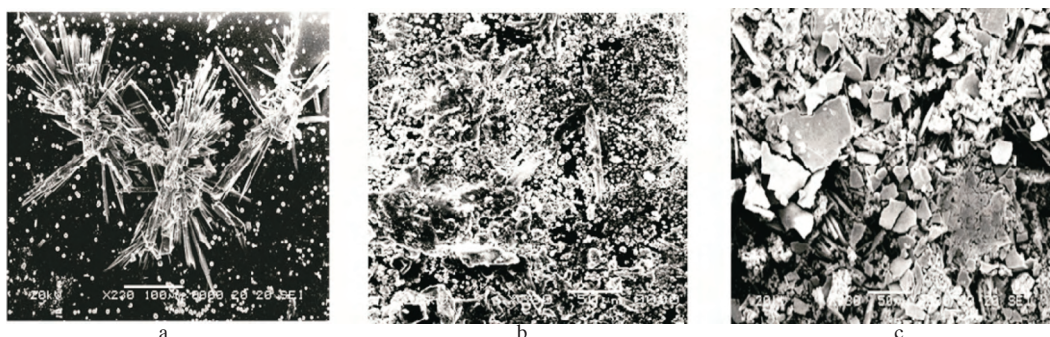
Figure 1. Effect of La doping on morphological features of different nanocrystalline CdS films with 0.2 ml TGM. Film structure of (a) undoped CdS; (b) CdS:NaF; and (c) CdS:NaF,La.
