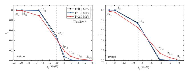
Figure 1. Upper panel: Occupation probabilities for neutrons as a function of temperature around the Fermi level. The calculations are performed using the finite temperature Hartree–Fock method at T = 0, 1, and 2 MeV for the <sup>56</sup> Fe nucleus. Lower panel: Same but for protons. The gray dashed lines indicate the Fermi level for neutrons and protons at zero temperature.
