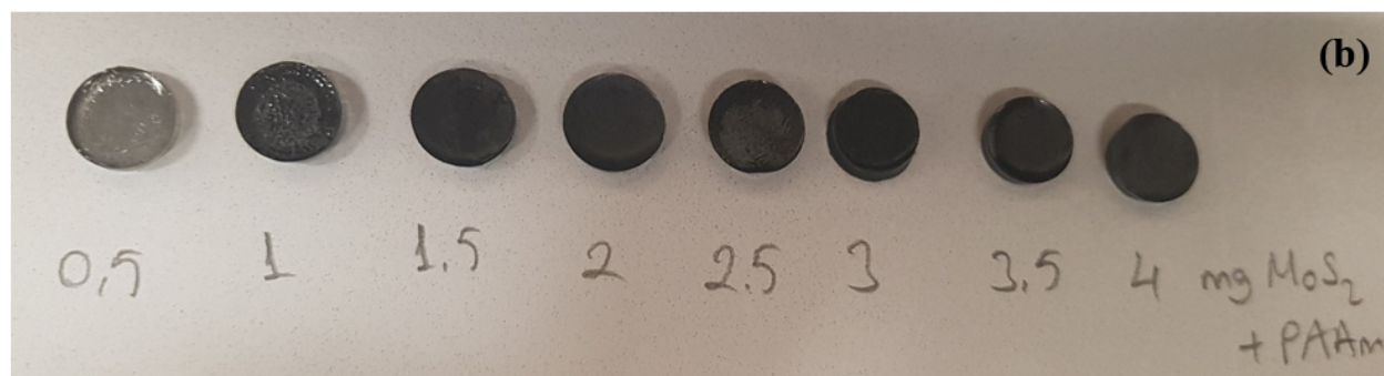
Figure 1. (a) Transmission-time graph of light through MoS 2 -PAAM solutions with different MoS 2 amounts inside a quartz cuvette. These spectra are used to obtain the sol-gel transition points of different polymer composites. (b) Dried MoS 2 -PAAM composite discs with various MoS 2 contents.
