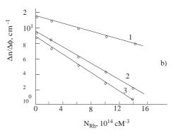
Figure 1.(a) The initial carrier removal rates dependence on initial concentration  $(n_0, cm^{-3}: 1-\sim 8.10^{15}; 2-\sim 1, 2.10^{15}; 3-\sim 8.10^{14}; 4-(0,2-8).10^{15})$  in  $n-Si\langle P, Rh\rangle$  (1-3) and  $n-S\langle P\rangle$  (4) after irradiation.
