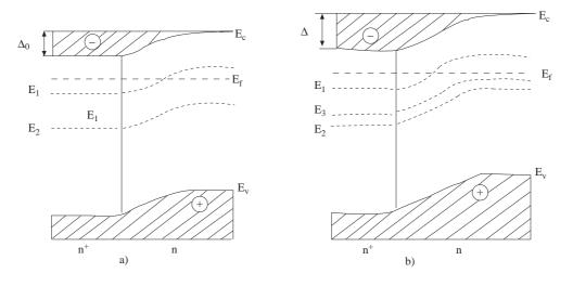
Figure 2. The barrier model of  $n^+$  and n areas occurrence in compensated silicon: a- before and b- after irradiation.
