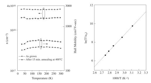
Figure 3. Results of the Hall-Effect measurements on the highly doped single GaInP layer (substrate is removed).
