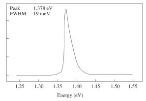
Figure 2. Room temperature photolumunescence spectrum for the bulk  $In_{0.1}Ga_{0.9}As$  sample
