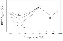
Figure 6. DLTS spectrum of a strained GaInP/In<sub>0.15</sub>Ga<sub>0.85</sub>As/GaAs sample with In-GaAs channel thickness of 150 Å
