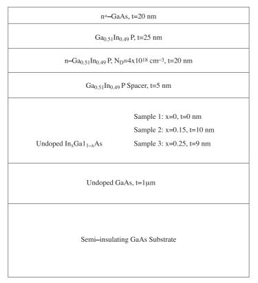
Figure 1. Grown MODFET structures
