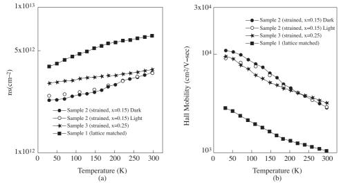
Figure 7. Results of the Hall-Effect measurements on the MODFET structures. (a) Sheet electron density, (b) Hall mobility
