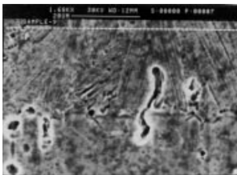
Figure 6. Scanning electron micrographs of porosities in welded zone.
