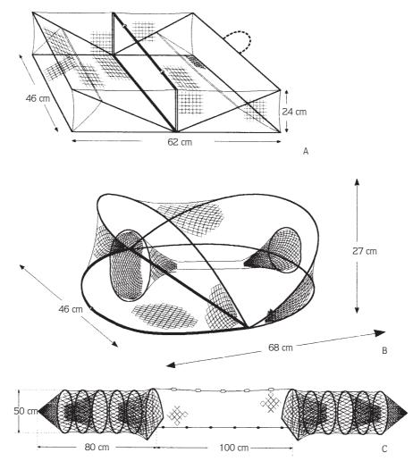
Figure 2. Diagram of a collapsible ellipsoid trap (CET) (A), a collapsible box type trap (CBT) (B) and a hoop net used to sample blue crab in Beymelek Lagoon, Antalya.
