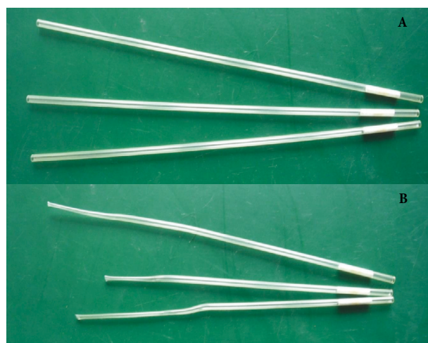
Figure 1. Types of cryodevices used in the study: A) conventional (French mini) straw and B) open pulled straw to achieve a diameter that was half of the original diameter.
