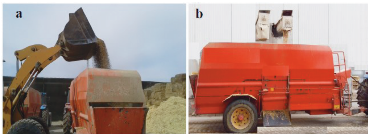
Figure 2. Two loading methods: (a) loading with loader, (b) spiral loading.
