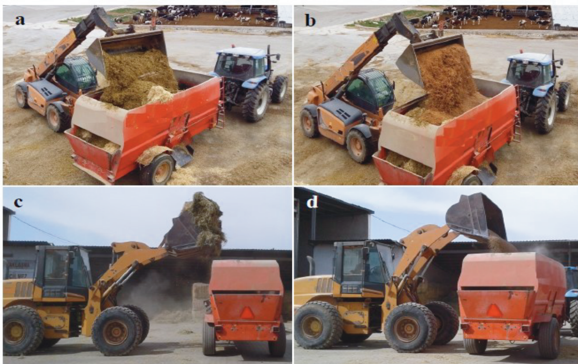
Figure 1. Examples of loading method according to physical properties of feedstuffs: (a) silage loading, (b) pulp loading, (c) rough loading, (d) concentrated loading.
