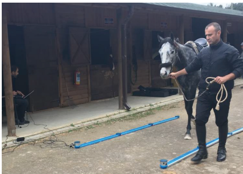
Figure 1. Measuring walking phases in a horse by OptoGait analysis system.
